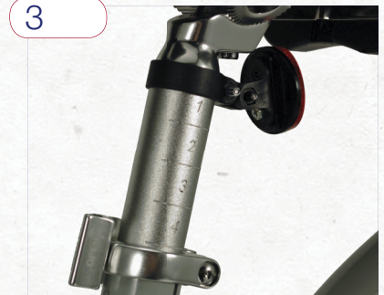
3 The seat post has graduated marks indicating its height. After adjustment, note your setting for future use.
